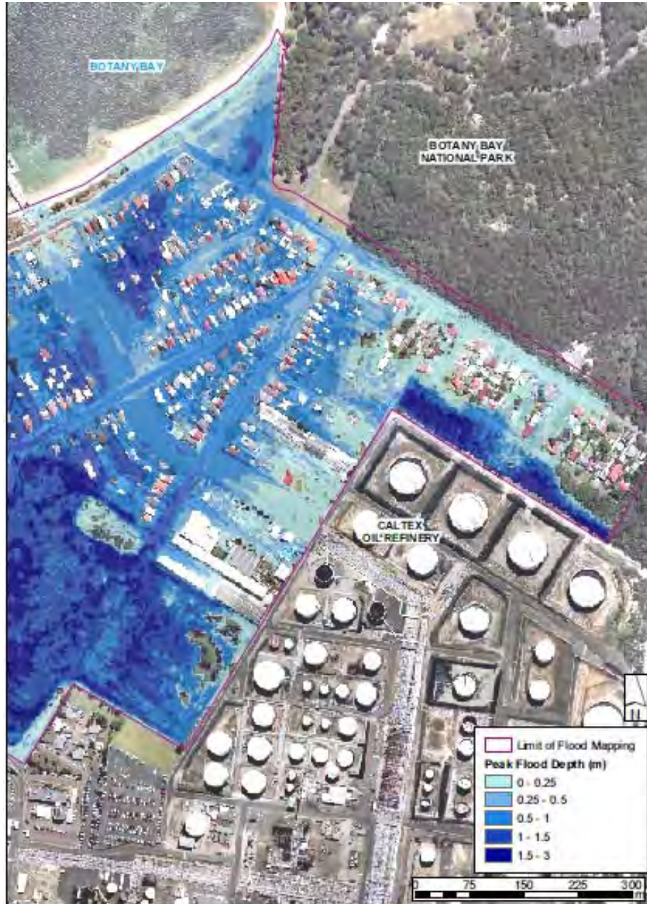
Figure 4-6 Peak Flood Depth 1% AEP Event Inset (WMAwater, 2009)
